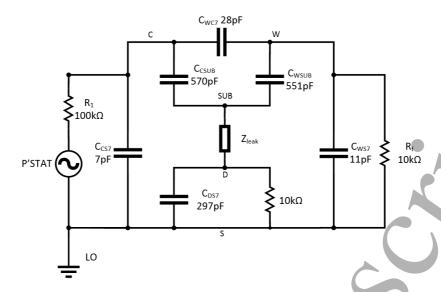
Figure 22. The SUB node has been added with a leakage impedance  $Z_{\text{leak}}$  through the encapsulation from the substrate to the PBS.
