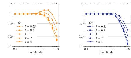
(a) G', normalised on its value at  $\gamma_0 = 0.1$  (b) G'', normalised on its value at  $\gamma_0 = 0.1$
