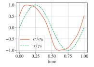
(a) A (normalised) nonlinear stress response,  $\sigma/\sigma_0$ , to oscillatory shear
