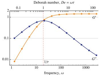
**Fig. 3.** A typical plot of *G'* and *G''* for a viscoelastic fluid—here, the Oldroyd-B fluid we investigate in Section 3.2—at different frequencies. The inverse of the frequency where the curves intersect,  $\tau$ , is described as the typical relaxation time of the fluid, and defines where the Deborah number,  $De = \omega \tau$ , is 1.
