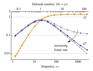
**Fig. 7.** The storage and loss moduli, *G*' and *G*", for an Oldroyd-B fluid. There is good agreement between the theoretical (dashed line) and experimental values. At high frequencies, measurements of *G*" at low frame rates (dotted line) diverge from the theoretical values, but increasing the frame rate (solid line) solves this. Parameters are as in Section 2.2.
