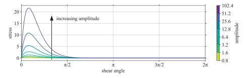
**Fig. 27.** Total system stress over the first unit of shear, where the Hookean dumbbells have zero natural length, starting with extensions of  $\Delta x = 20$ . Here the spring force is k = 2. In particular, notice that the stress response is no longer periodic.
