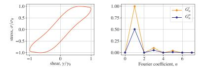
(b) The Lissajous curve for the stress re- (c) Taking the Fourier transform of the stress sponse displays its nonlinearity by its non-elliptical shape. (c) Taking the Fourier transform of the moduli  $G'_n$  and  $G''_n$ .
