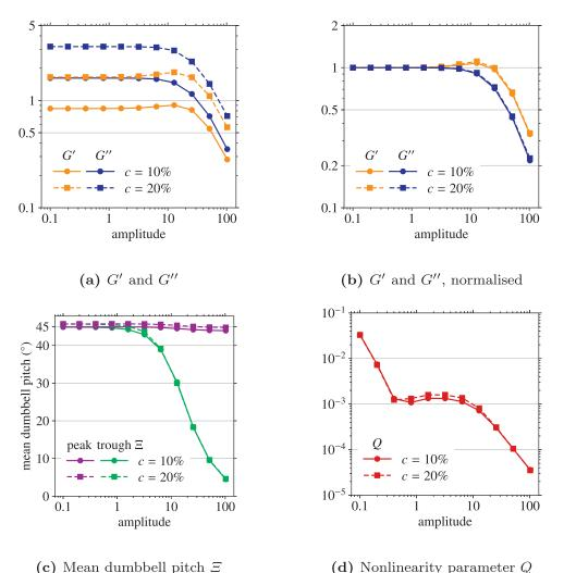
Fig. 18. An amplitude sweep of our Hookean dumbbell solution at two different dumbbell concentrations, at De = 0.56.
