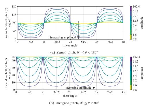
**Fig. 14.** Mean dumbbell pitch for Hookean dumbbells (k = 2, L = 20) over two cycles of shear at different amplitudes. The arrow points in the direction of increasing amplitude, from  $\gamma_0 = 0.8$  to 102.4, doubling each time. System details as in Section 4.2.
