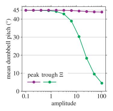
**Fig. 15.** Measuring the heights of the peaks and troughs in fig. 14b across amplitudes, we can describe the alignment of the dumbbells.
