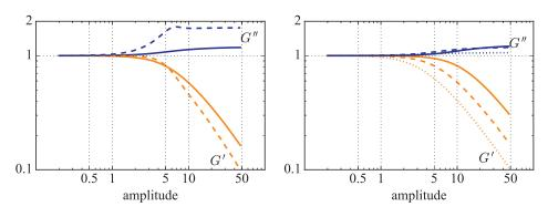
(a) Normalised G' and G'' at frequencies (b) Normalised G' and G'' with maximum of  $\omega = 10\pi/3$  (solid lines) and  $20\pi/3$  dumbbell extensions of  $\ell = 20$  (dotted lines). dumbbell ines), 40 (dashed lines) and 80 (solid lines).
