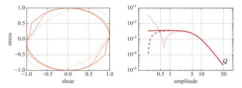
(b) Lissajous plot at amplitudes of  $\gamma_0 =$  (c) Nonlinearity parameter Q at increasing reso-0.1 (dotted line), 12.8 (dashed line), lution: 250 timesteps per oscillation (dotted line), 2500 (dashed line) and 25,000 (solid line)
