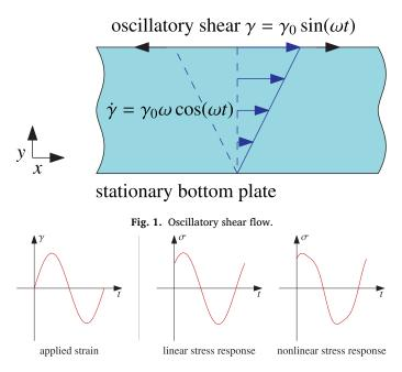
**Fig. 2.** A linear and nonlinear stress response to an oscillatory shear over time. For SAOS, we expect the former, but for LAOS, we expect the latter.
