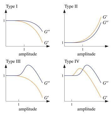
**Fig. 12.** Four types of behaviour for normalised *G*' and *G*'' in a LAOS amplitude sweep, reproduced from Hyun et al. [12]: Type I, strain thinning; Type II, strain hardening; Type III, weak strain overshoot; Type IV, strong strain overshoot.
