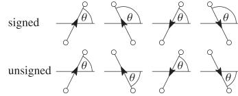
Fig. 13. Two ways of measuring alignment for dumbbell vectors  $\Delta x$  pointing in different directions: signed, where  $0^{\circ} \le \theta < 180^{\circ}$ , and unsigned, where  $0^{\circ} \le \theta < 90^{\circ}$ .
