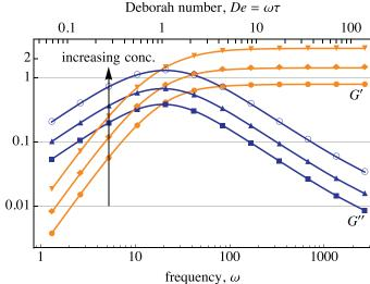
**Fig. 8.** The storage and loss moduli, *G*' and *G*'', for Hookean dumbbells at concentrations of 10%, 20% and 40%. Higher concentrations lead to proportionally higher readings. The relaxation time,  $\tau$ , is unaffected by the increase in concentration, providing the same mapping from frequency to Deborah number for all concentrations.
