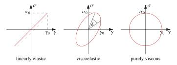
**Fig. 4.** Lissajous curves for a linearly elastic solid, viscoelastic fluid, and purely viscous fluid. The eccentricity of the orbit gives an indication as to the balance between viscous and elastic effects. By fitting an ellipse to the data, accurate measures of  $\sigma_0$  and  $\delta$  can be found.
