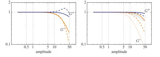
(a) Normalised G' and G'' at frequencies (b) Normalised G' and G'' with maximum of  $\omega = 10\pi/3$  (solid lines) and  $20\pi/3$ (dashed lines).
