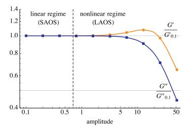
**Fig. 6.** An amplitude sweep of our Hookean dumbbell solution: for a fixed frequency ( $\omega = 10\pi/3$ , De = 0.56), at low amplitudes, G' and G'' (here, normalised by their values at amplitude 0.1) are independent of amplitude, but at higher amplitudes, this changes. This sweep test allows us to find the linear regime region.
