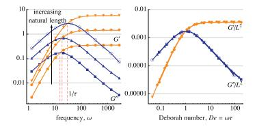
**Fig. 10.** Left: The storage and loss moduli, G' and G'', for Hookean dumbbells show a strong dependence on the natural dumbbell length, here 10, 20, and 40 units. Increasing the dumbbell length leads to increases in the measurements. **Right:** Plotted against Deborah number and scaled by  $L^2$ , the different graphs of G' and G'' collapse onto each other.
