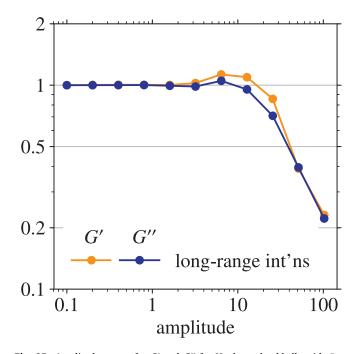
**Fig. 25.** Amplitude sweep for *G'* and *G''* for Hookean dumbbells with De = 0.56, where particles interact through far-field hydrodynamics using the Rotne–Prager–Yamakawa tensor. The *G'* bump is visible. Sweep undertaken at reduced resolution of 120 RK4 timesteps per oscillation, compared to the usual 1200, due to increased computational intensity.
