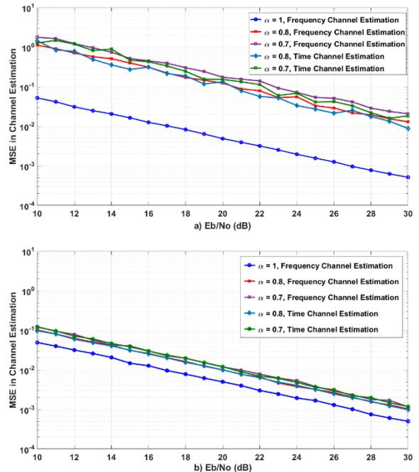
Fig. 2: MSE of time-domain and frequency-domain channel estimation. (a) Random pattern. (b) Same QAM symbol pattern.
