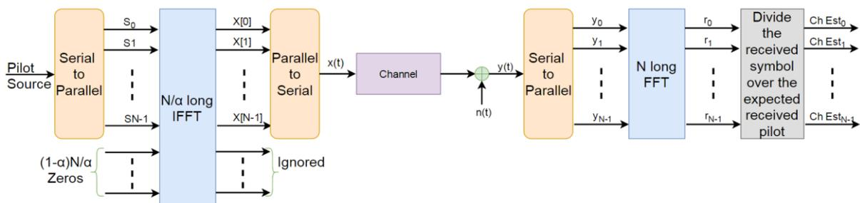
Fig. 1 SEFDM transceiver with channel estimation block
