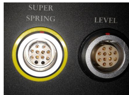
Figure 8.9 Faulty pins in the super-spring LEMO socket on the SIMX
