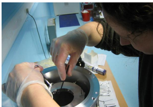
Figure 8.2 Releasing the dropping chamber snubber lock nuts
