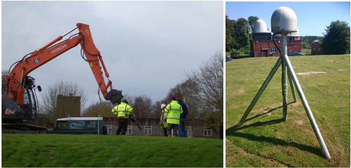
Figure 11.4 The UK's Ordnance Survey reference receiver 'HERO'. The photograph on the left shows the installation of the monument, the photograph on the right is the installed unit.
