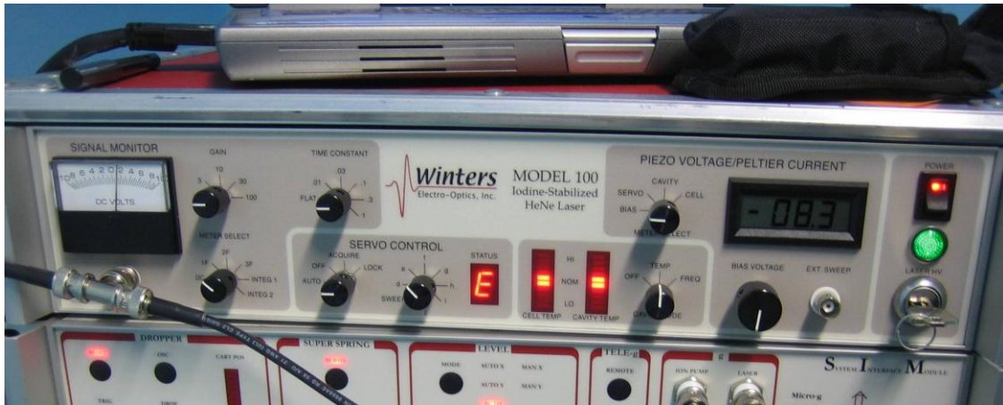
Figure 2.9 WEO-100 Laser control electronics within the gravimeter electronics rack
