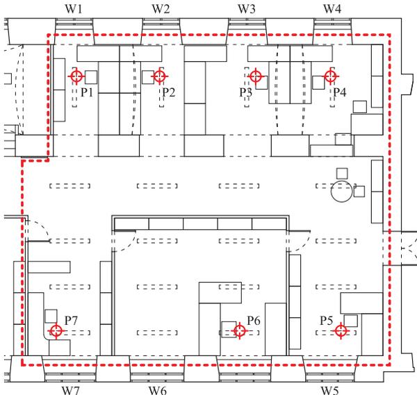
Figure 1: Schematic illustration of the office area, observed occupants and operable windows
