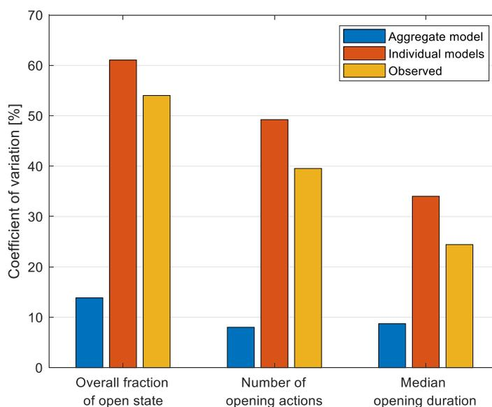
Figure 6: Coefficient of variation of the overall fraction of open state, number of opening actions, and median opening duration across the occupants obtained from observations, aggregate and individual window operation models
