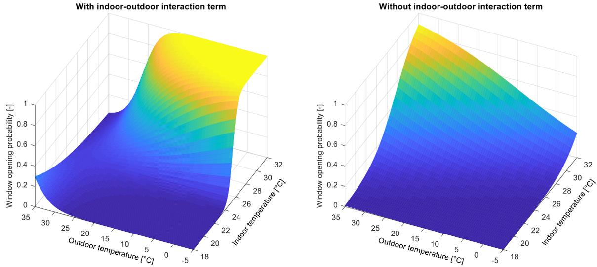
Figure 4: Three-dimensional surface plot of the individual window operation model W5 with indoor-outdoor interaction term (left) in comparison with the fitted model without interaction term (right).
