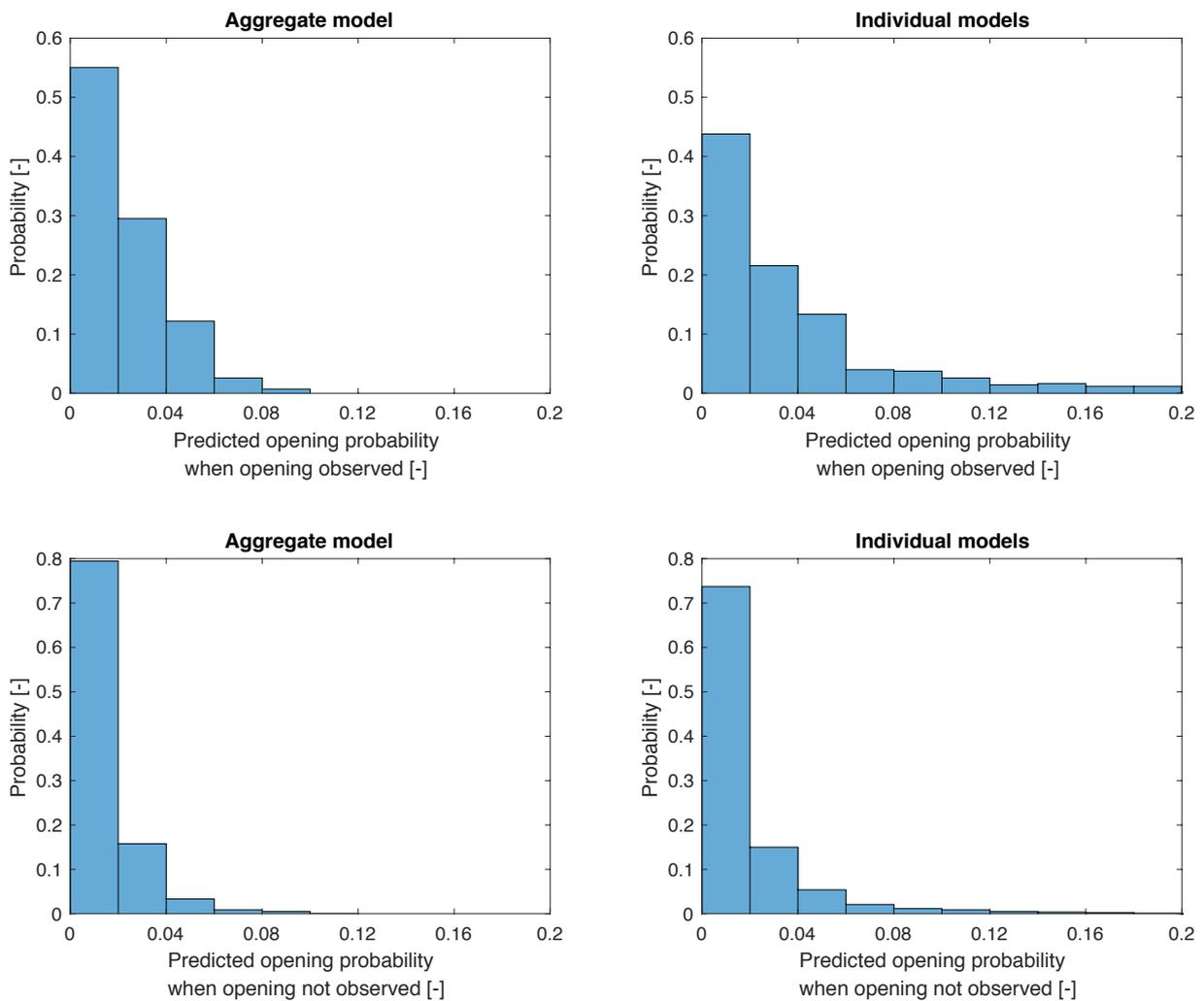
Figure 5: Histograms of predicted window opening probabilities by aggregate (left) and individual (right) models for the intervals where the closed windows were opened (top) and for the intervals where the windows remained closed (bottom).
