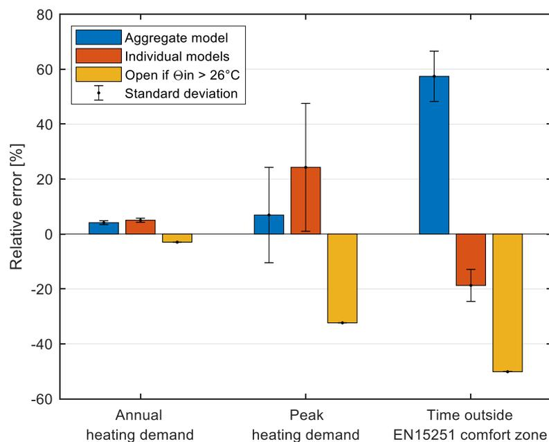
Figure 7: Relative error of the performance indicators obtained from the building model with aggregate and individual window operation models as well as a simple non-probabilistic model
