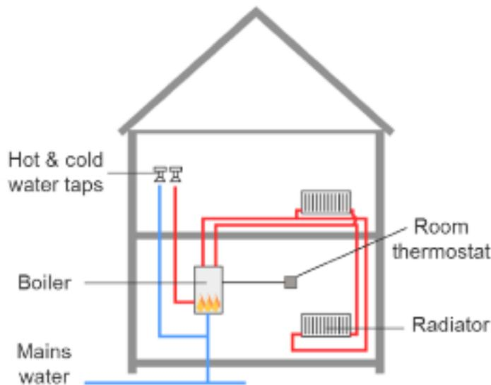
Figure 1: Schematic of typical combi boiler heating and hot water system.
