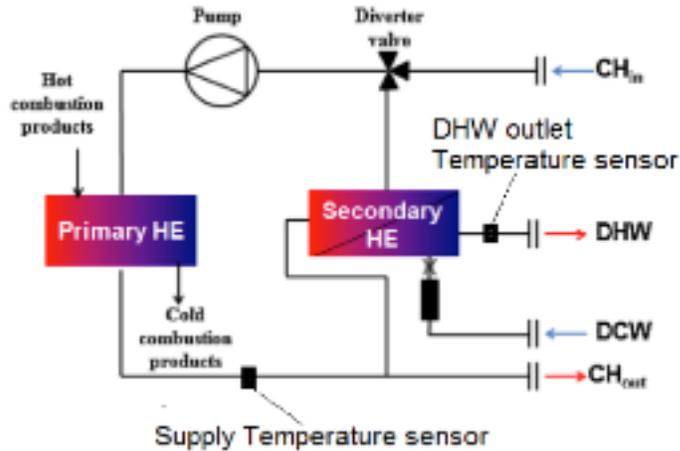
Figure 2. Combination boiler schematic. (CH: Central Heating, DHW: Domestic Hot Water, DCW: Domestic Cold Water, HE: Heat Exchanger)
