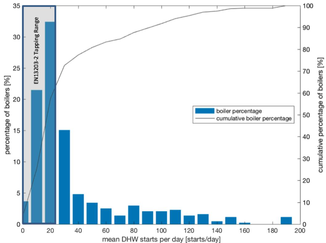
Figure 7: Histogram of average DHW starts per day (EN13203-2 Tapping range shaded in grey)
