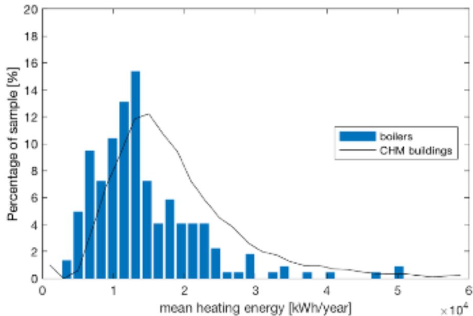
Figure 5: Annual building space heating energy demand derived from boiler data compared to modelled space heating demand of the English housing stock (Field data & CHM <sup>41</sup>)
