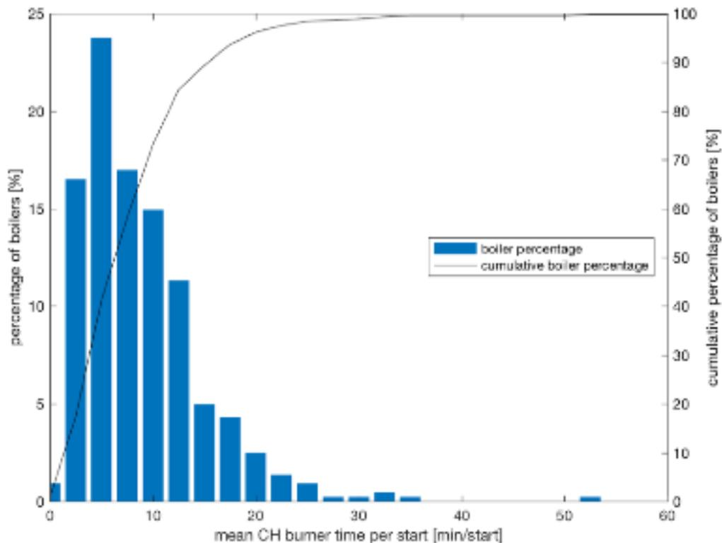
Figure 9: Histogram of mean CH runtime per start
