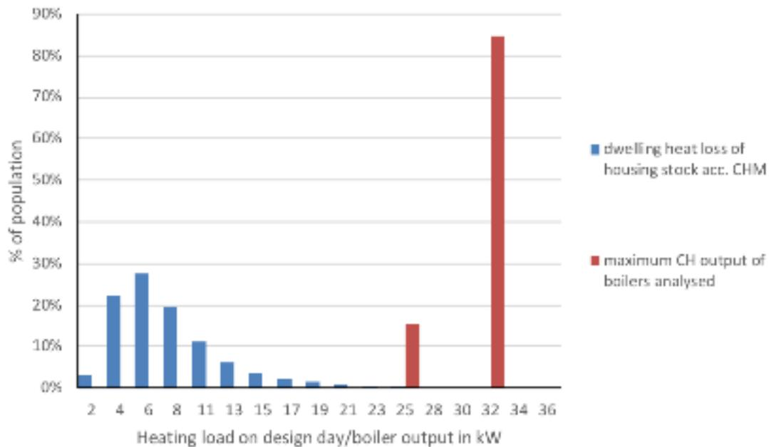
Figure 4: Distribution of English housing stock building heat loss on design day as predicted by the Cambridge Housing Model <sup>41</sup> compared to the maximum CH output of the boilers analysed in this paper.
