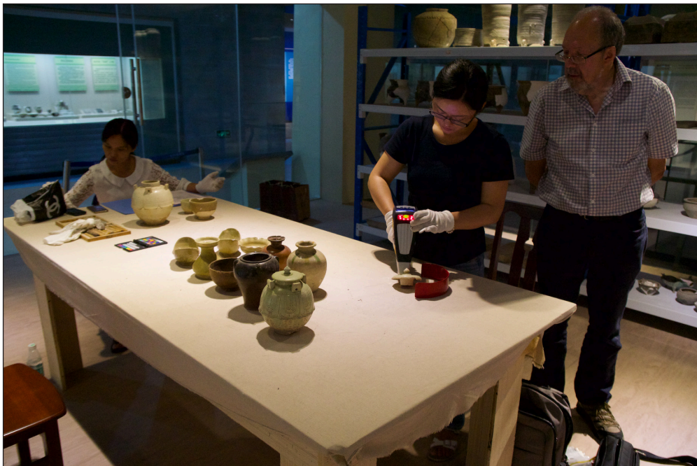
Figure 2: Analysing ceramic samples with pXRF at Anyang Museum in Henan Province (Photo Lihua Shen).
