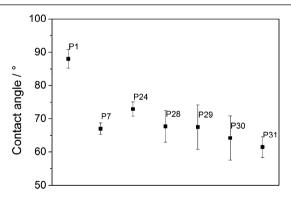
**Figure 4.** Contact angles for P1, P7, P24, P28, P29, P30, and P31 against water.  $P7^{51}$  is a copolymer of phenylene and dibenzo[b,d]-thiophene, included for comparison.
