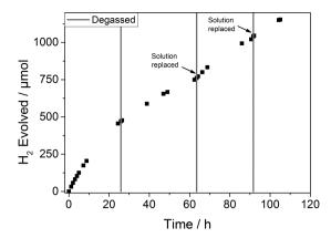
Figure 5. Extended hydrogen evolution experiment for P28 under visible light ( $\lambda$  > 420 nm) from a H<sub>2</sub>O/MeOH/TEA mixture for a total of 105 h. The solution was intermittently degassed, and after 63 and 92 h the H<sub>2</sub>O/MeOH/TEA mixture was replaced.
