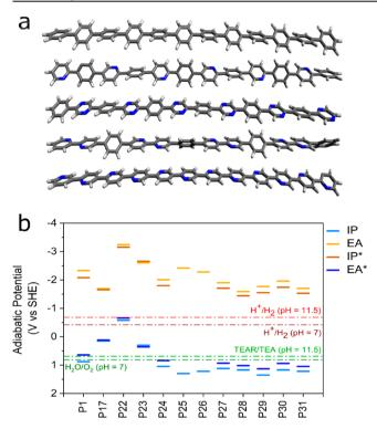
Figure 3. (a) B3LYP/DZP optimized structures of oligomer models representing polymers P1, P24, P28, P30, and P31. (b) Predicted charge carrier (IP, EA) and exciton (IP\*, EA\*) potentials of polymer materials considered. For guidance, various potentials for solution reactions are also given: reduction potential for hydrogen and oxidation potential for water at pH7; reduction potential for hydrogen and oxidation potential for the SED (TEA) at pH 11.5.
