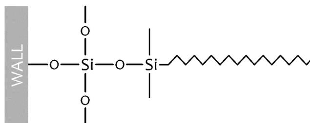
**Figure 3.1 Chemical structure of the stationary phase.**
