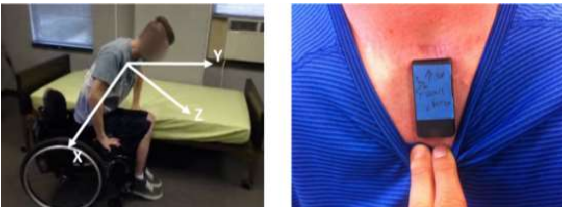
Figure F-0-2 Orientation of the accelerometer's axes in respect to the body during wheelchair transfers and position of the accelerometer on the participant's sternum
