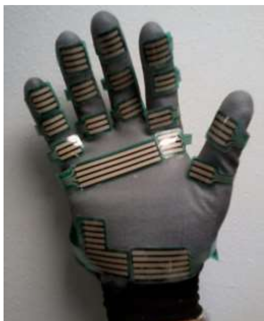
Figure 5-1 Position of the force sensitive resistors on the palm of the hand
