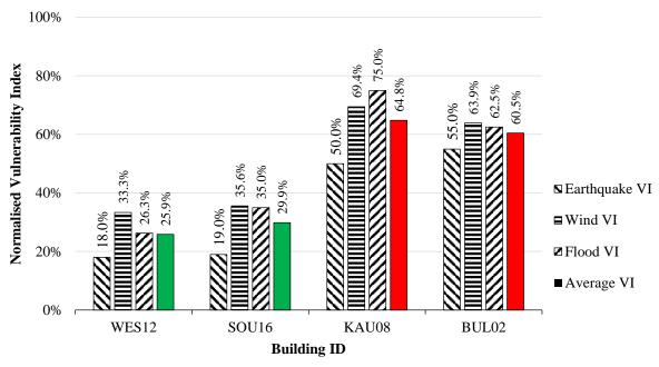
Figure 7. Evaluated vulnerability index of buildings based on the different hazards
