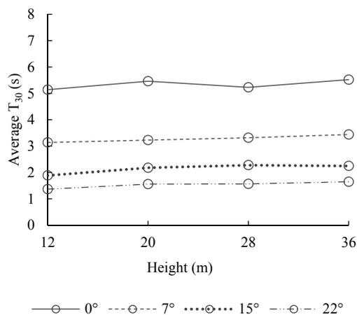
Figure 21. Average  $T_{30}$  for a slope of a single pitched skylight with an aspect ratio of 3
