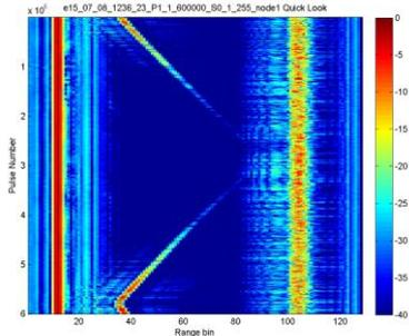
Figure 4: RTI plot of walking human target
