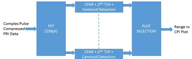
Figure 7: Signal Processing Chain
