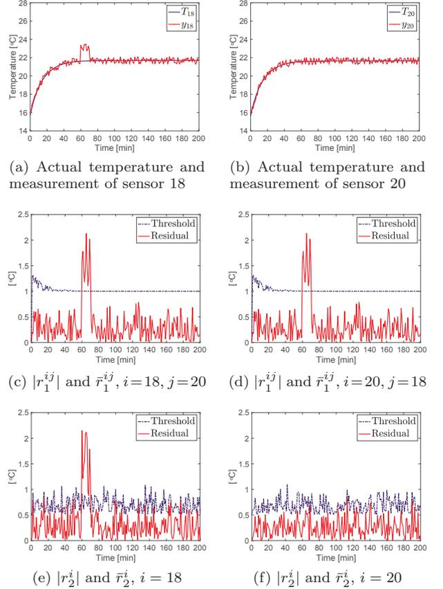
Fig. 3. Comparison between sensor 18, affected by an intermittent fault  $f_{(18)}(t) = 1.5 \cdot [u(k - k_{f_{18,1}}) - u(k - k_{f_{18,2}})]$ ,  $k_{f_{18,1}} = 60$  min,  $k_{f_{18,2}} = 70$  min, and the healthy sensor 20.
