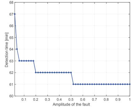
Fig. 4. Detection time vs. fault amplitude ( $c$  parameter) for single linear degrading faults,  $k_f = 60$  min.
