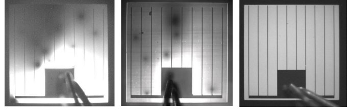
Figure 11: Representative electroluminescence images of the regular (left) and QD (middle) thin-film cells in comparison to that of a substrate based cell (right). The thin-film cells showing point defects and misfit dislocation lines typically require currents in the 40-80 mA range while the substrate based cells showing homogeneous luminescence require currents in the 0.5-5 mA range to obtain an image.
