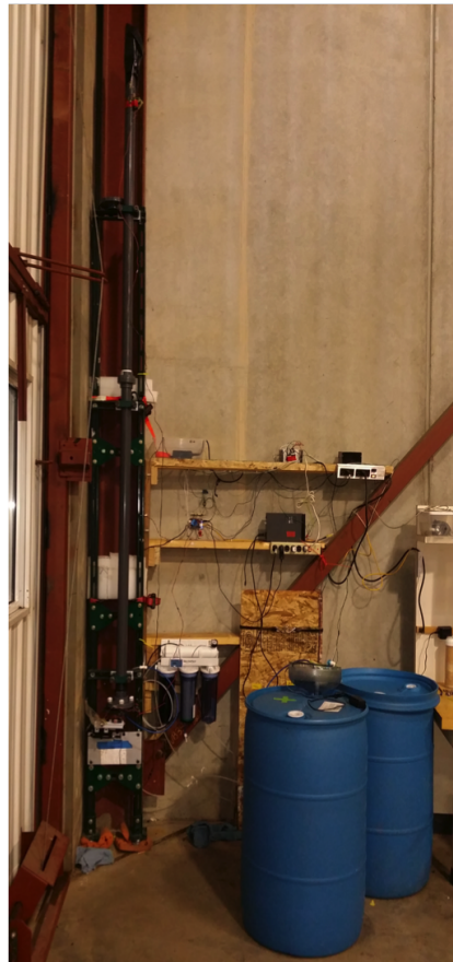
Figure 1: Left: schematic showing the key features of the water column (lengths in mm) and right: photograph of the setup in the laboratory showing the column (left), the filters(centre) and the barrel (forefront right).
