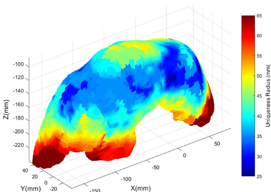
registration in the landmarks used for TRE assessment. The aim here is to test how well our uniqueness map predicts the amount of acquired data required for a reliable registration. Therefore, the radius  $R_S$  at which GO-ICP successfully aligns the LUS data to the CT should be similar to the radius  $R_U$  predicted by the framework given the point-based reference standard alignment.
