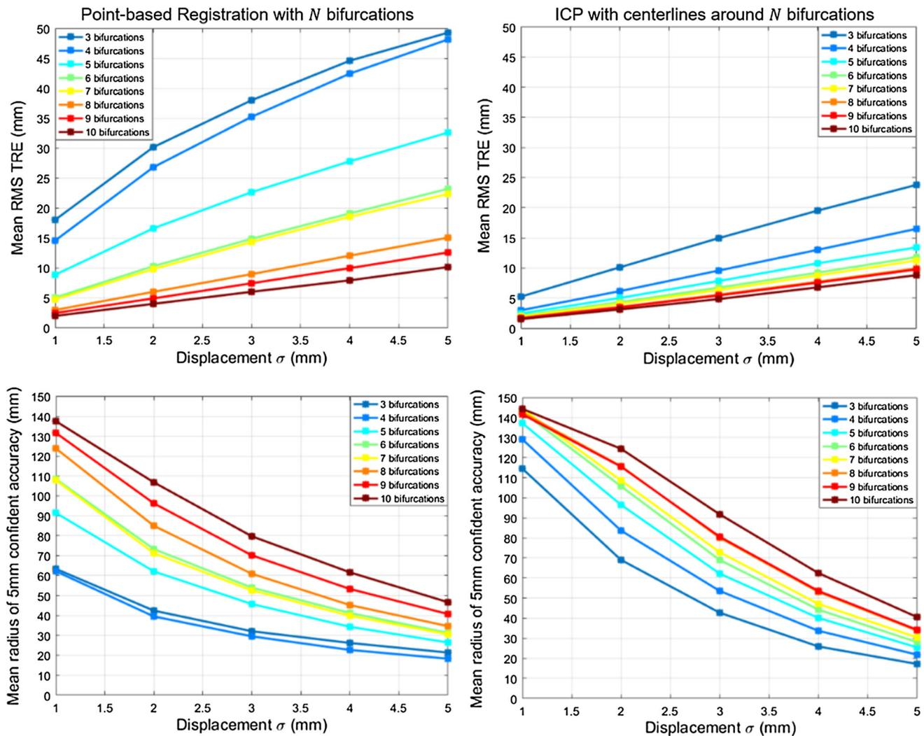
**Fig. 2** Accuracy results on vessel bifurcations after running results of the first experiment. The top row presents the RMS of the TRE on bifurcations; the bottom row represents the radius where accuracy is better
