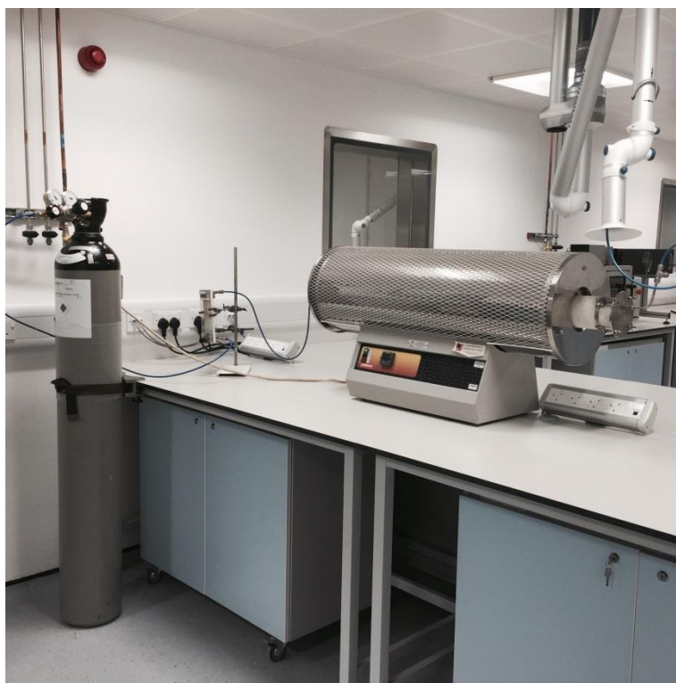
Figure 10: Experimental set up for carbonisation
