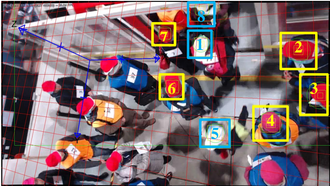
Figure 3-11: Example of Petrack used to track the position of A_i ( i = 3 ) when R = 1
