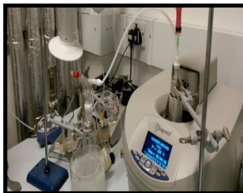
Figure 5-1 Experimental set-up of microwave-assisted synthesis of pre-PGS in single mode Discover SP system.
