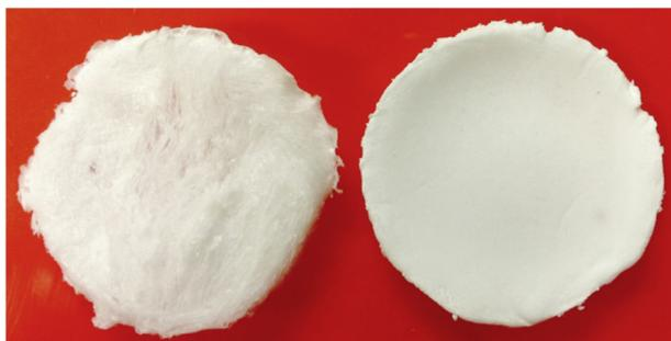
Fig. 1 – AB-PEO composites: AB30 (left) and AB70 (right).
