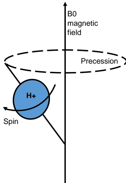
**Figure 4.1** Proton spin and precession within the magnetic field generated by an MRI scanner
