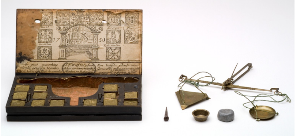
FIGURE 8.3 Balance used for the weighing of coins, eighteenth century. IMAGE USED BY THE KIND PERMISSION OF MUSEUM BOERHAAVE, LEIDEN.
