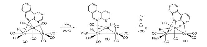
Scheme 1. Reactivity of  $[Os_3(CO)_9(\mu_3-\eta^1,\kappa^1-C_{13}H_8N)(\mu-H)]$  towards PPh<sub>3</sub> [8].
