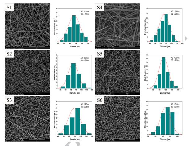
Fig. 3 SEM images and diameter distributions of the fibers. The scale bar in the SEM
