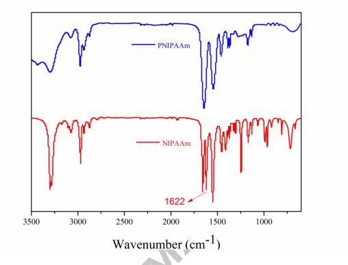
Fig. 2 FTIR spectra of PNIPAAm and NIPAAm
