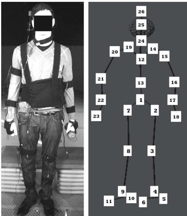
Fig. 4.4. A participant wearing the Animazoo IGS-190 sensor system (Left) and the 26 tracked anatomical joints (labelled from 1 to 26) tracked by the system (Right)
