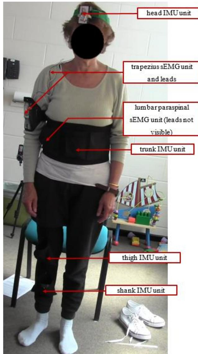
Fig. 7.13. The placement of 4 IMU units and 2 sEMG units of the prototype on participant P4-3 in the data collection study
