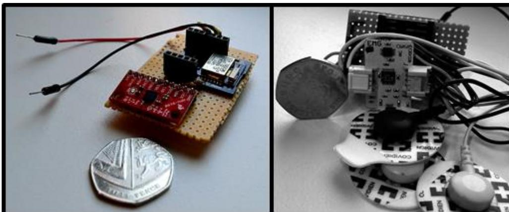
Fig. 7.1. Left - an IMU sensing unit of the MOVES-PC prototype; Right - an sEMG sensing unit of the prototype
