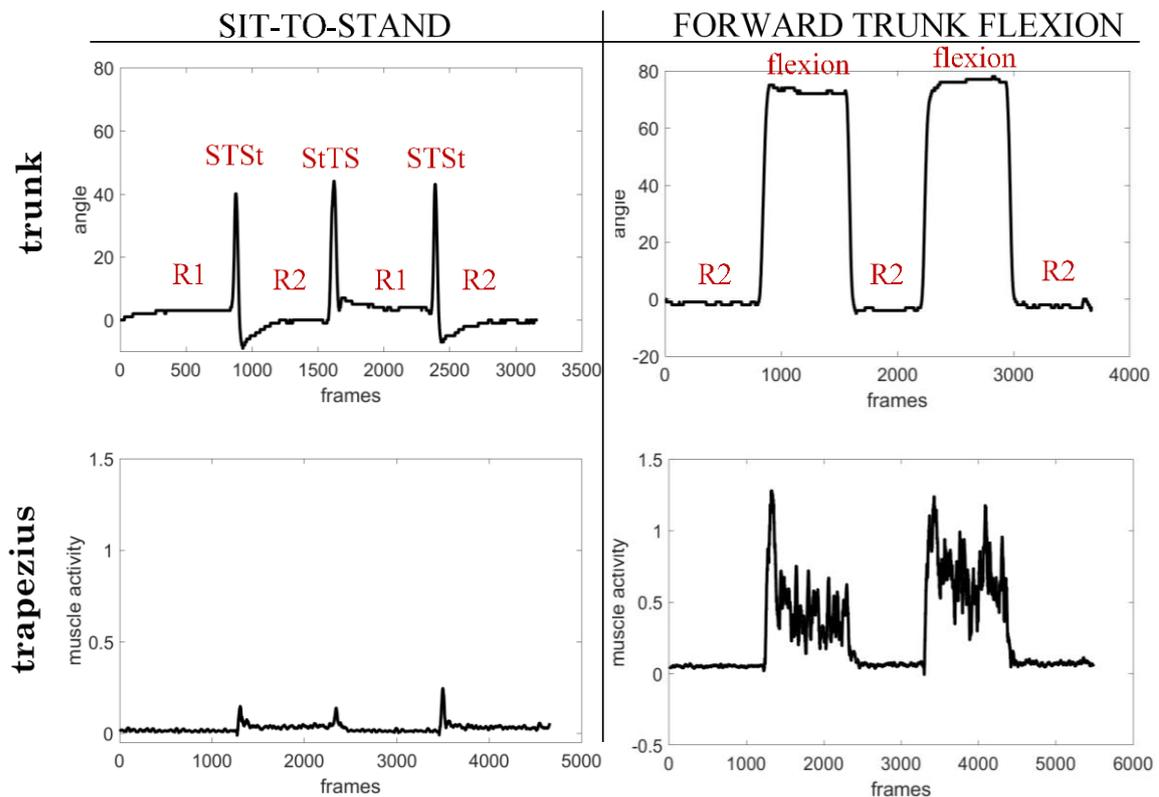
Fig. 7.10. Trunk flexion/extension (Top) and concomitant activity of the trapezius (Bottom) during the Sit-to-Stand (Left) and Forward Trunk Flexion (Right) for participant P1-2. *STSt* = *sit-to-stand*; *StTS* = *stand-to-sit*; *R1* = *sitting*; *R2* = *standing*
