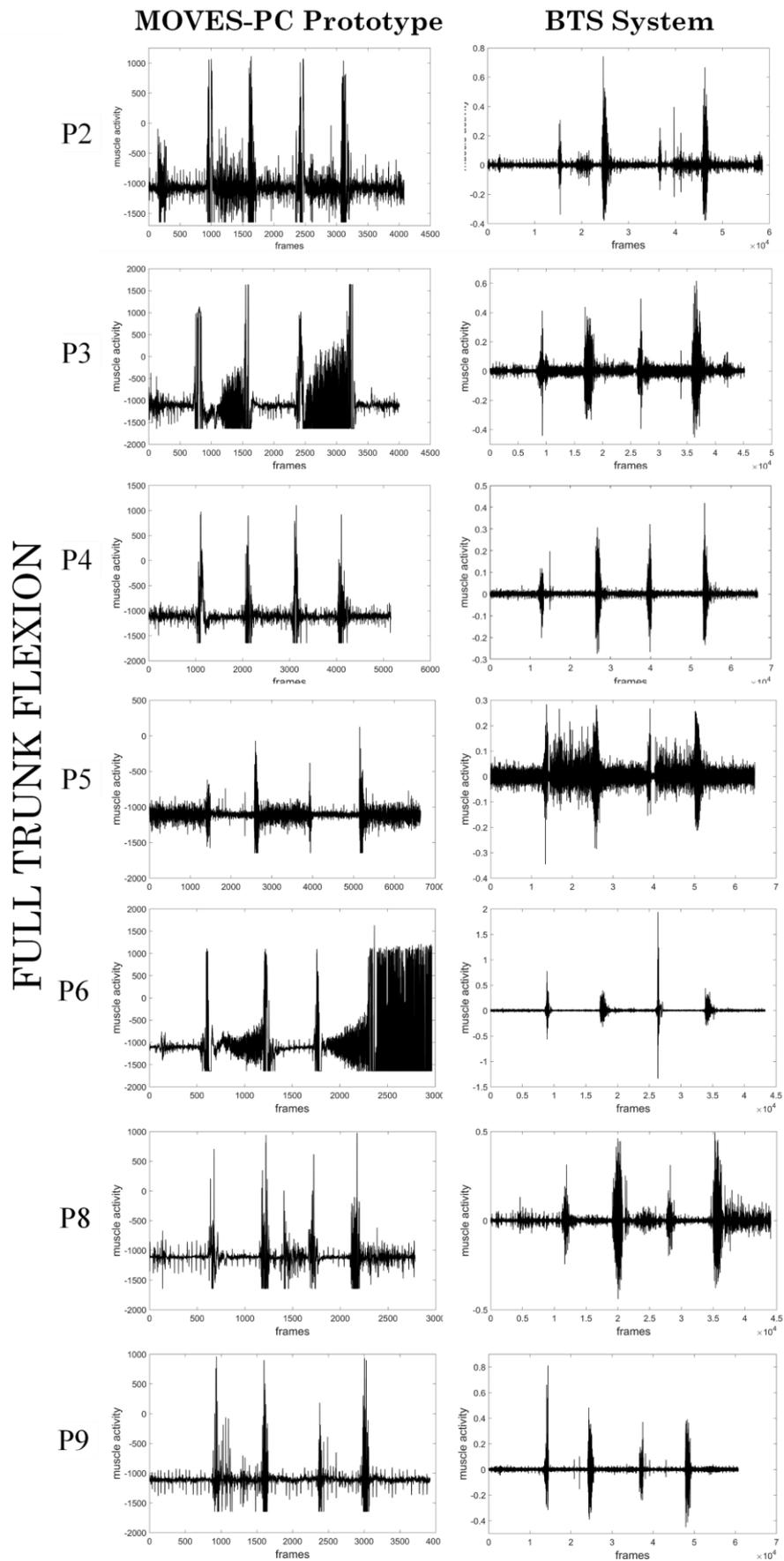
Fig. 7.9. Activity of the lumbar paraspinal of each of 7 participants captured using the low-cost MOVES-PC prototype (Left) and the expensive BTS system (Right)
