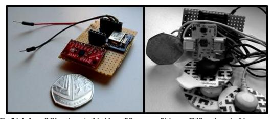
Fig. 7.1. Left - an IMU sensing unit of the Moves-PC prototype; Right - an sEMG sensing unit of the prototype
