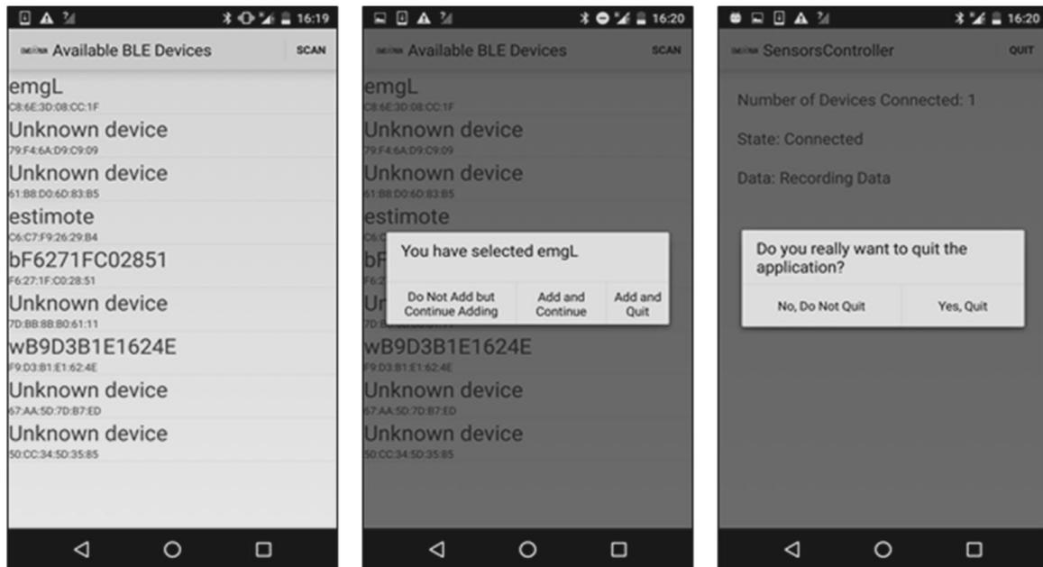
Fig. 7.2. MOVES-PC mobile application screenshots: Left - the list of BLE devices available during a scan; Middle - dialog in connecting to one of the sensing units of the prototype; Right - dialog in terminating a recording session
