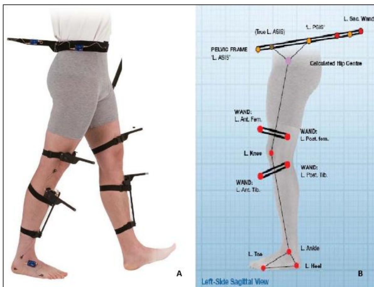
Figure 5.5 Image indicates active marker placement: [A] A participant with markers placed on his legs, feet and pelvic. [B] Schematic of marker placement that form different segments.
