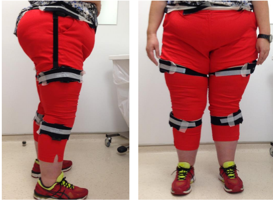
Figure 4-2: Positioning of the sensors on pelvis, thighs and calves
