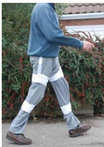
Figure 3-2: Volunteer walking with the IMUs strapped to the thigh and shank (adapted from McCarthy et al., 2013)
