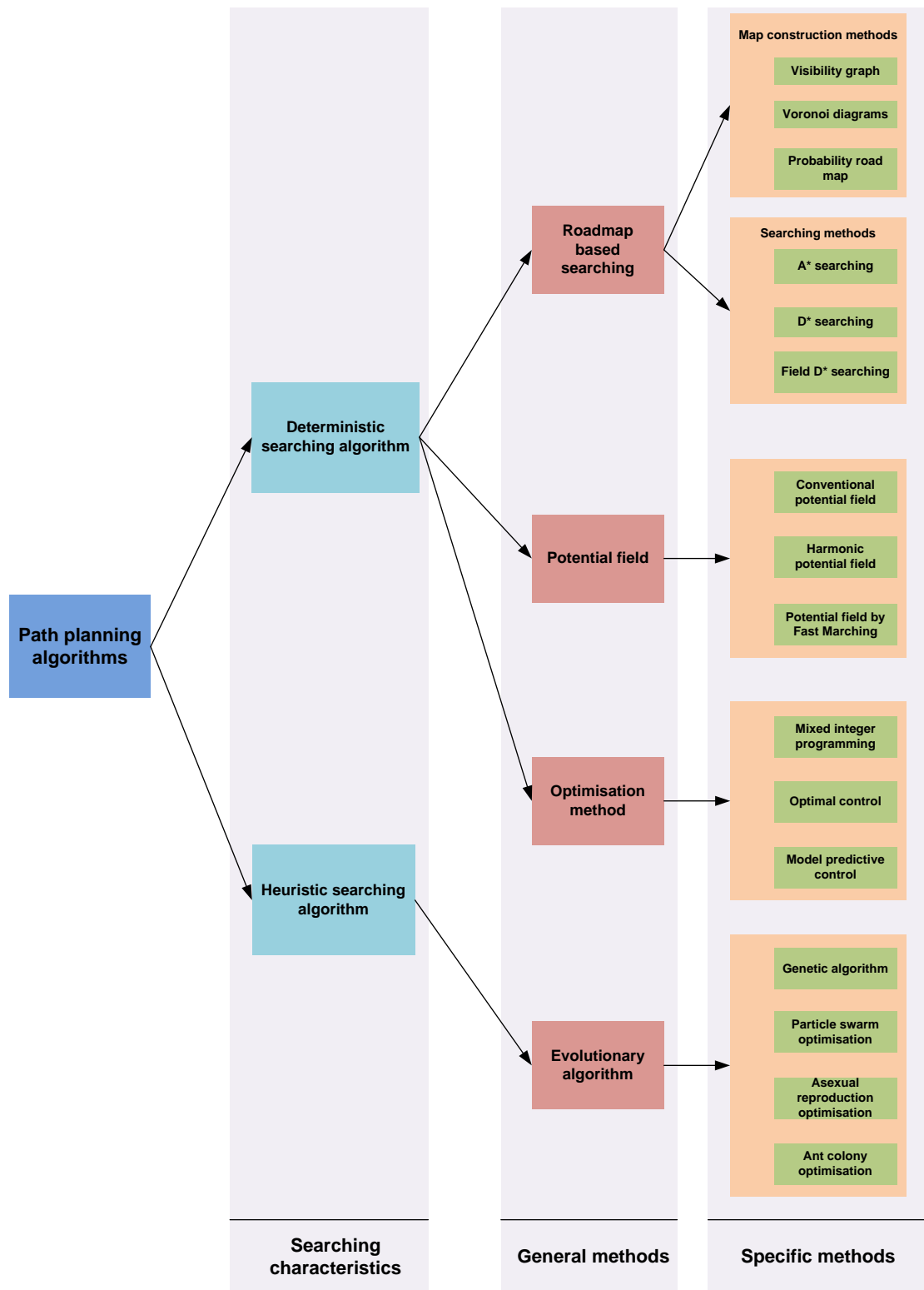
Fig. 13: The categorising of path planning algorithms based upon deterministic and heuristic approaches.
