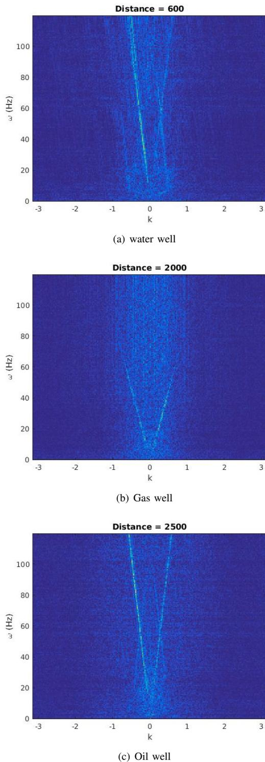
Fig. 4. A sample of the V-shape angle in each well pipe at different distance along the pipeline.
