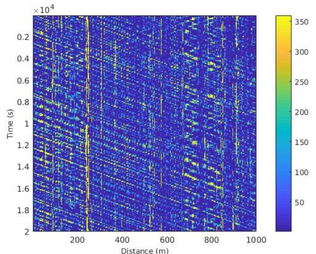
Fig. 1. Sample of acoustic raw data in time-distance domain.
