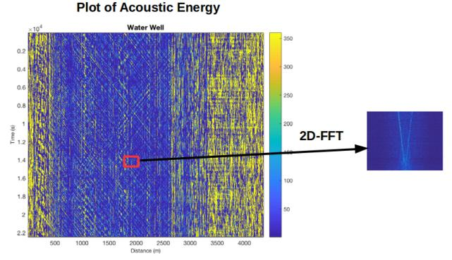
Fig. 3. A sample of V-shape image in oil dataset which obtained after applying 2D-FFT to time-distance acoustic data.
