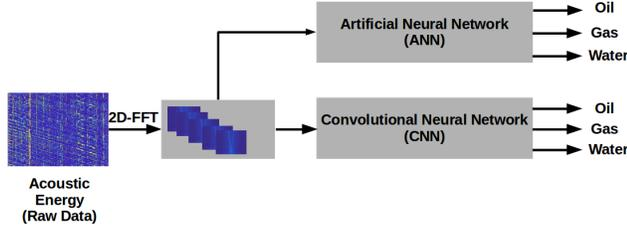
Fig. 2. Overview diagram for classifying fluid flow regime in oil, gas and water well pipes. Acoustic data are converted from time-domain to frequency-wave number domain using 2D-FFT.
