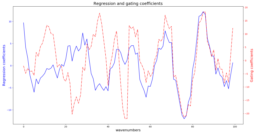
Figure 10: PLSR coefficients (6 factors) and gating function coefficients for protein calibration.
