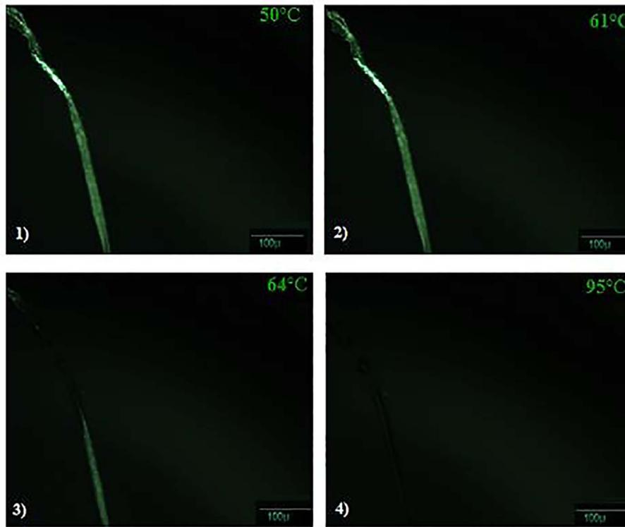
**Fig. 4a.** Melting of PEO fiber bundle without progesterone (stages 1–4 representing temperatures 50 °C, 61 °C, 64 °C and 95 °C) visualised by hot-stage microscopy. At stage 4, the PEO fiber had melted completely.
