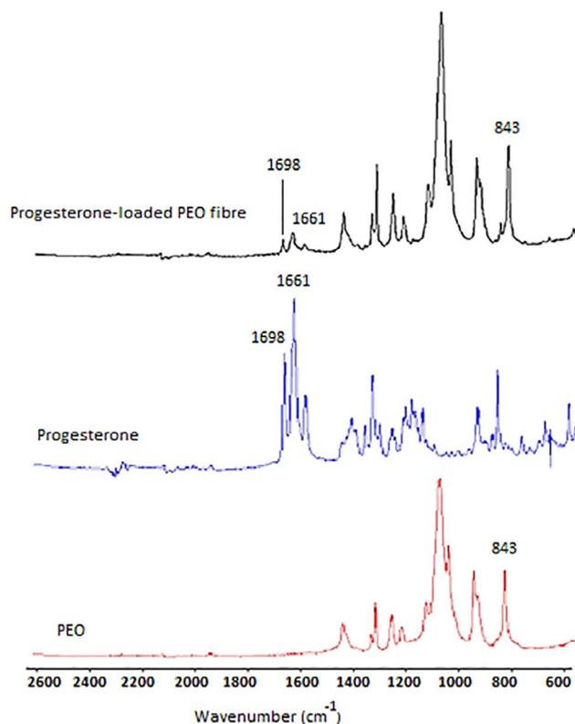
Fig. 3. TR-FTIR spectra of PEO and progesterone in the 600–2600  $\text{cm}^{-1}$  region showing characteristic peaks and that of drug-loaded PEO (with initial solvent loading of 5% progesterone) fibers confirming the presence of encapsulated progesterone.
