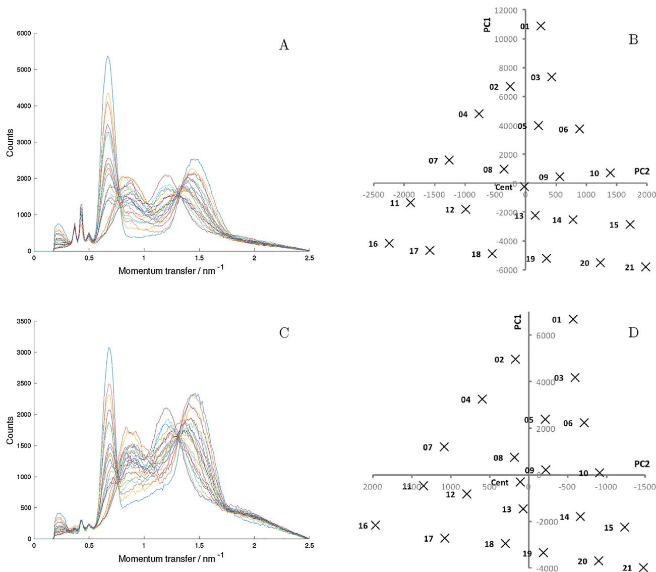
**Fig. 5.** Plots (A) and (B) show the raw data of the samples of unpackaged tablets and the corresponding scores plots of the first two PCs for all samples from the left to right, respectively. Plots (C) and (D) show the raw data of the samples of packaged tablets and the corresponding scores plots of the first two PCs for all samples from the left to right, respectively. Pure sample profiles are also plotted separately in Supplementary Data 1.
