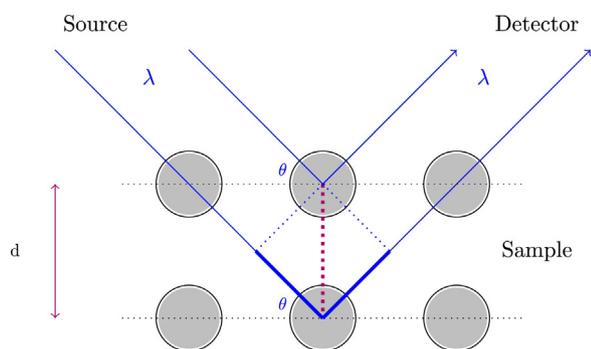
**Fig. 1.** X-ray incident on two parallel planes at an angle  $\theta$ , with photon wavelength  $\lambda$  and planar spacing  $d$ . The thicker ray line represents the additional path length traversed in a reflection from the lower plane which, for a coherent scattering event, is an integer multiple of the X-ray wavelength, satisfying Bragg's law.
