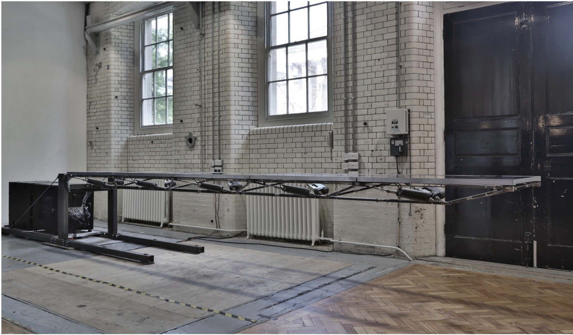
Figure 1. Adaptive truss prototype, University College London Structures Laboratory.
