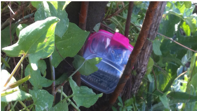
Figure 3: A light sensor placed in the community garden to measure light levels
