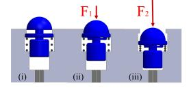
**Figure 3.** Compression of the tactile element: (i) no force is applied, the tactile element is not compressed; (ii) small force ( $F_1$ ) is applied, ortho-planar spring only is compressed; (iii) large force ( $F_2$ ) is applied, both ortho-planar and linear springs are compressed.
