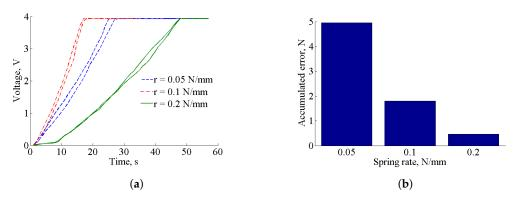
**Figure 9.** Performance of the hysteresis for liner springs. (a) Hysteresis curves for force elements with different spring rates; (b) Accumulated errors for hysteresis loops for force elements with different spring rates.
