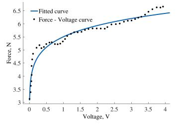
**Figure 10.** Calibration curve for tactile elements with spring rate 0.2 N/mm-fitted line and force-voltage response.
