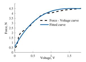
**Figure 11.** Calibration curve for a hybrid tactile element employing two springs: ortho-planar spring and linear spring. The two springs were chosen based on the described experimental study: the linear spring has a constant of 0.2 N/mm and the height of the leg of the ortho-planar is 0.6 mm.
