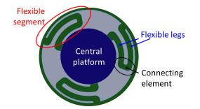
**Figure 4.** Ortho-planar spring: bottom view of the ortho-planar spring showing the structure of the flexible segments.
