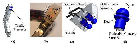
**Figure 1.** Fibre optical fingertip tactile sensor: (**a**) design of the fingertip fiber optical sensor; (**b**) photo of sensor integrated with prototype fingertip, dimensions are shown in mm; (**c**) section view of the fingertip sensor: fingertip tactile array; (**d**) hemispherical dome-shaped element.
