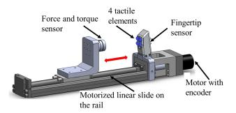
**Figure 8.** Calibration setup comprised from the linear motorized slide to implement repetitive movement, and a force and torque sensor to measure control forces.
