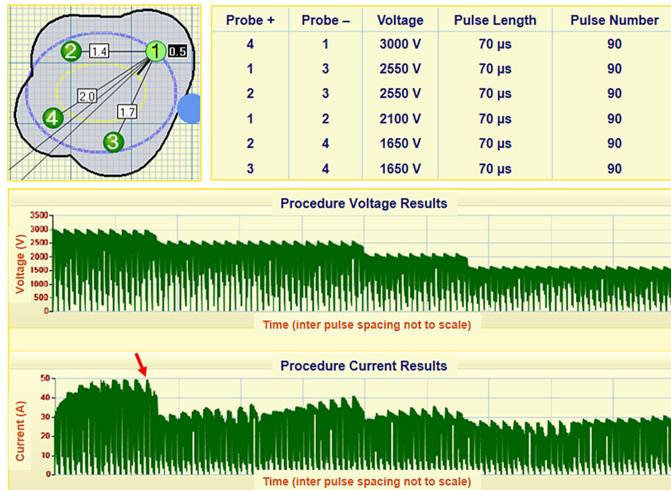
FIG. 1. Electrode positioning and pulse protocol for patient P2. The graphical user interface calculates the inter-electrode spacing and the necessary voltage to achieve 1500 V/cm. Voltage and current are reported following treatment. The NanoKnife delivers pulses in groups of 10 before recharging the capacitor bank, as evident by the periodic drop in voltage and current. The red arrow indicates the current matched during the derivation of the conductivity functions.
