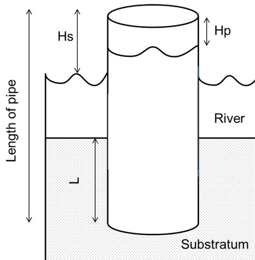
**Figure 2.11** Variables used to calculate VHG at an upwelling site in which  $H_s$  is the distance from the top of the piezometer to the river surface;  $H_p$  is the distance from top of the piezometer to the surface of the water within the piezometer;  $L$  is the depth of the pipe in the substratum and  $VHG = (H_s - H_p)/L$  (Dahm and Valett, 1996).
