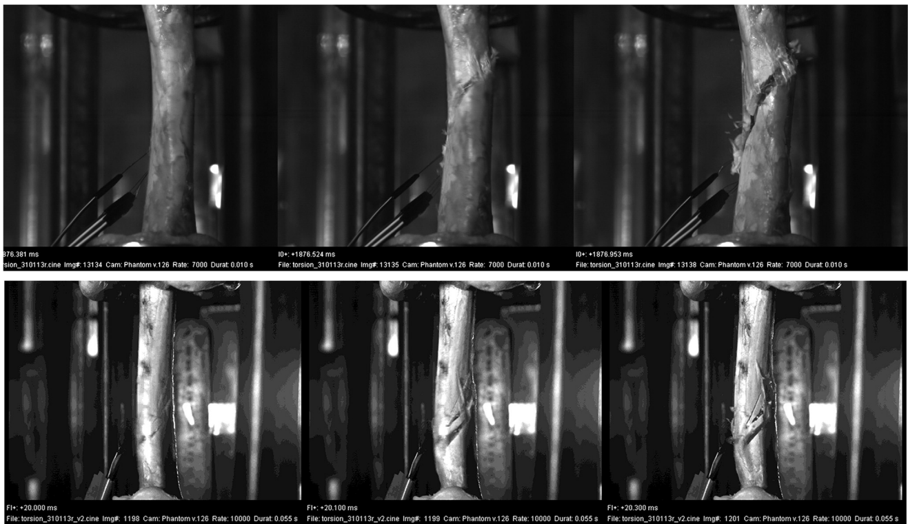
Fig. 6. (Top) The progression of a 'clean' spiral fracture that took place over 0.572 ms in three video frames (frame rate of 7000 fps) for a tibia tested at the low strain rate (specimen TS4). The fracture angle occurred at approximately 30°. (Bottom) The progression of spiral fractures with several fracture paths of about 45° (specimen TF4) acquired at 10,000 fps.
