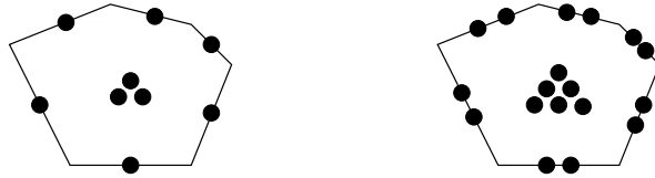
FIG. 4.1. Uncut hexagonal cell. Left: k = 0 ; right: k = 1 . Each dot attached to a geometric entity (face or cell) symbolizes one degree of freedom (not necessarily a pointwise evaluation).
