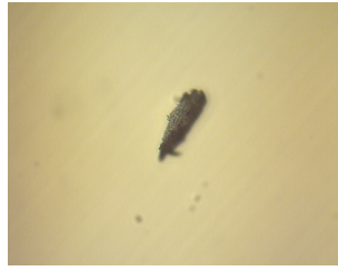
Figure 7.4: Surface defect (pit) under optical microscopy.
