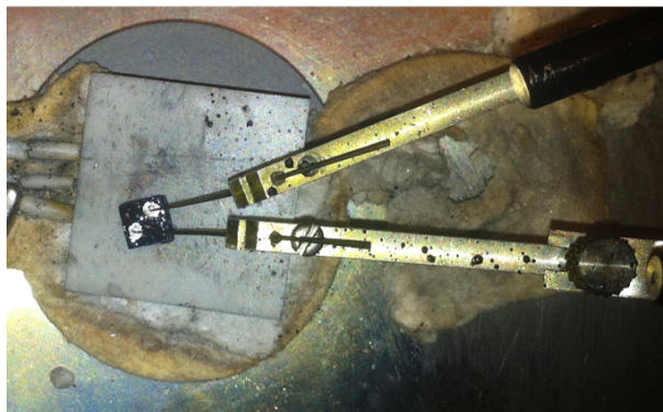
Figure 5.1: Image of the CNT-epoxy sample under impedance spectroscopy.
