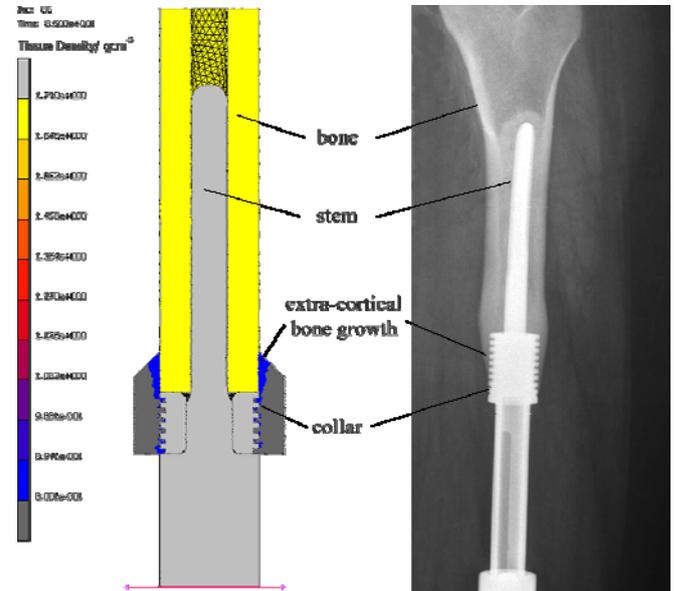
**Figure 1:** Left: Predicted bone growth (blue) with elastic modulus of approximately 2 GPa around an implanted grooved collar (light grey) and cortical bone shaft (yellow). Right: Good correspondence with X-ray results taken 12 years after implant insertion, where there was adventitious bone formation and good osteointegration with the HA-coated collar.
