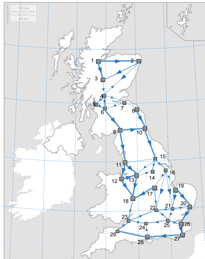
Fig. 8. Electricity flow in the best deterministic case at t=6 .
