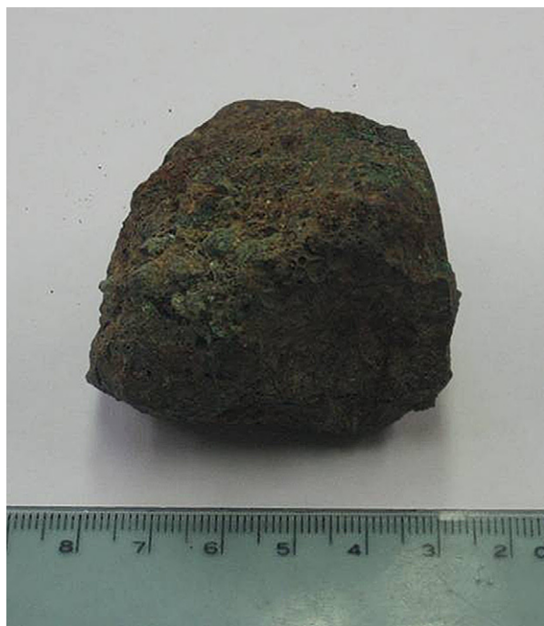
Fig. 12. Photograph of the slag (S120) found together with the crucible discussed here at the bottom of the 1976 test trench on the North Flat at Tepe Hissar. Note the large, massive form of this iron-rich and heavy slag, which is unlikely to have been produced in the small crucibles usually associated with Chalcolithic smelting practices.
