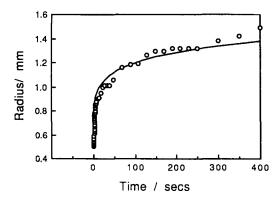
Fig. 5. Re-plot of some of the Ni-11P on nickel data shown in Fig. 3. The line is a plot of the de Gennes relationship with m = 3 and  $K_m = 603 \times 10^{-34} \text{ m}^{10} \text{ s}^{-1}$  and  $R_0 = 5 \times 10^{-4} \text{ m}$ .
