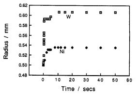
Fig. 4. Radii of drops of copper on nickel and tungsten.
