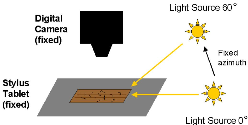
Image: Figure 2: A Diagram of the image capture system. Whilst the elevation of the light source changes around the tablet, the camera and tablet remain stationary.
