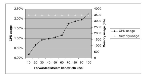
Figure 5.6: UTG selective forwarding memory and CPU usage
