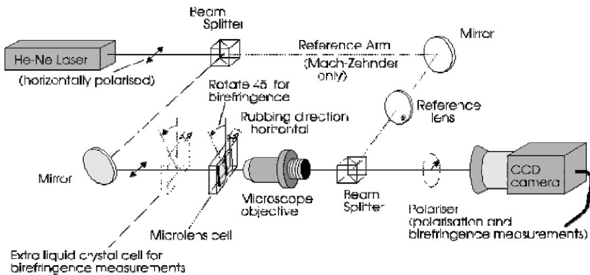
Figure 2: The interferometer setup used as a Mach-Zehnder, for birefringence measurements and for polarisation measurements
