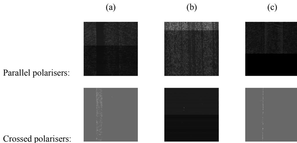
Figure 3: The cylindrical lenses (original (a), strip electrode (b) and electrode-on-top (c)) as seen through crossed and parallel polarisers, input polariser parallel to rubbing direction with 8V applied.
