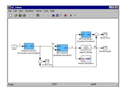
Figure 4: The control model of a generic agent in Matlab-Simulink.
