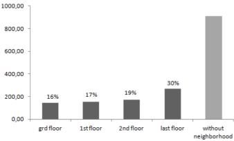
Figure 3: Access to solar radiation in kWh/m² per year and percentage of solar radiation available at this solar orientation for each façade with neighbourhood, EnergyPlus calculations.
